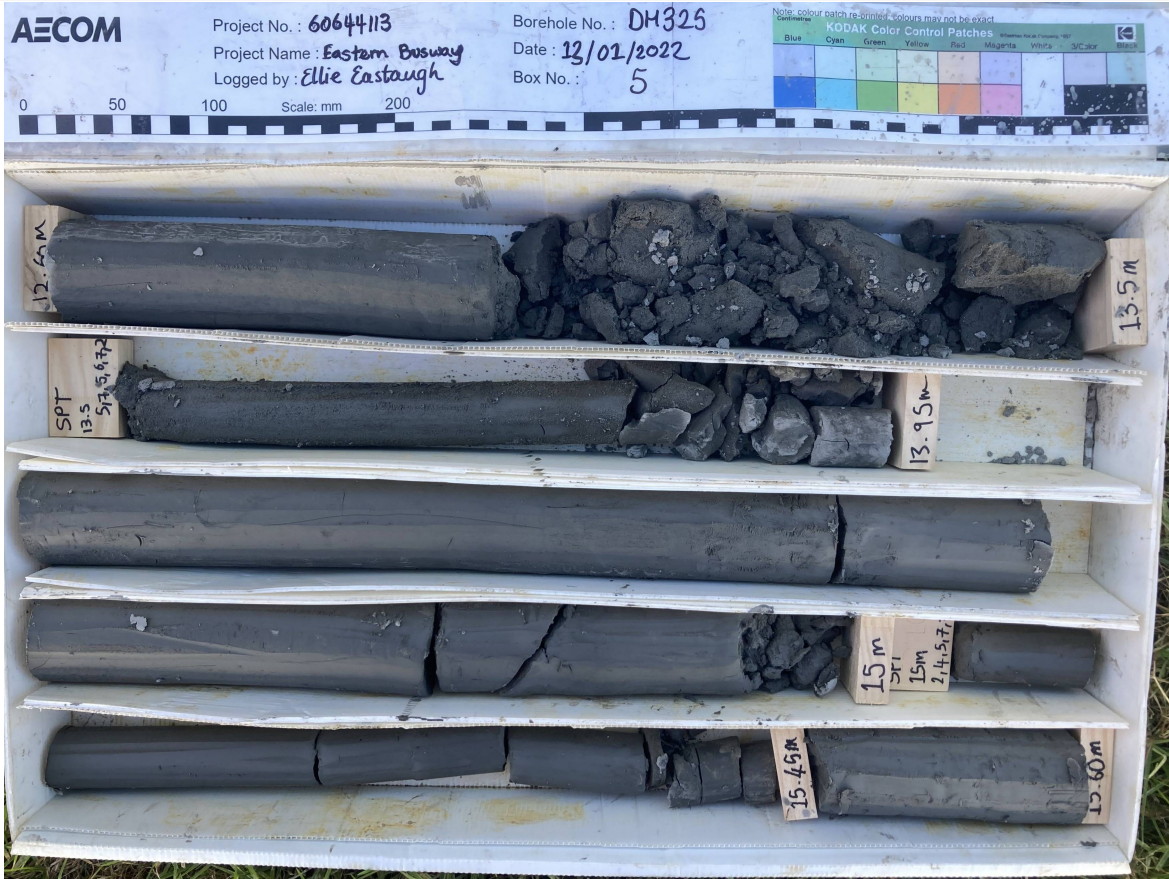
Box: 5 of 9 - Depth: 12.60m to 15.60m of 28.50m Date Drilled 12/01/2022 to 14/01/2022 - Date Photographed: 13/01/2022
