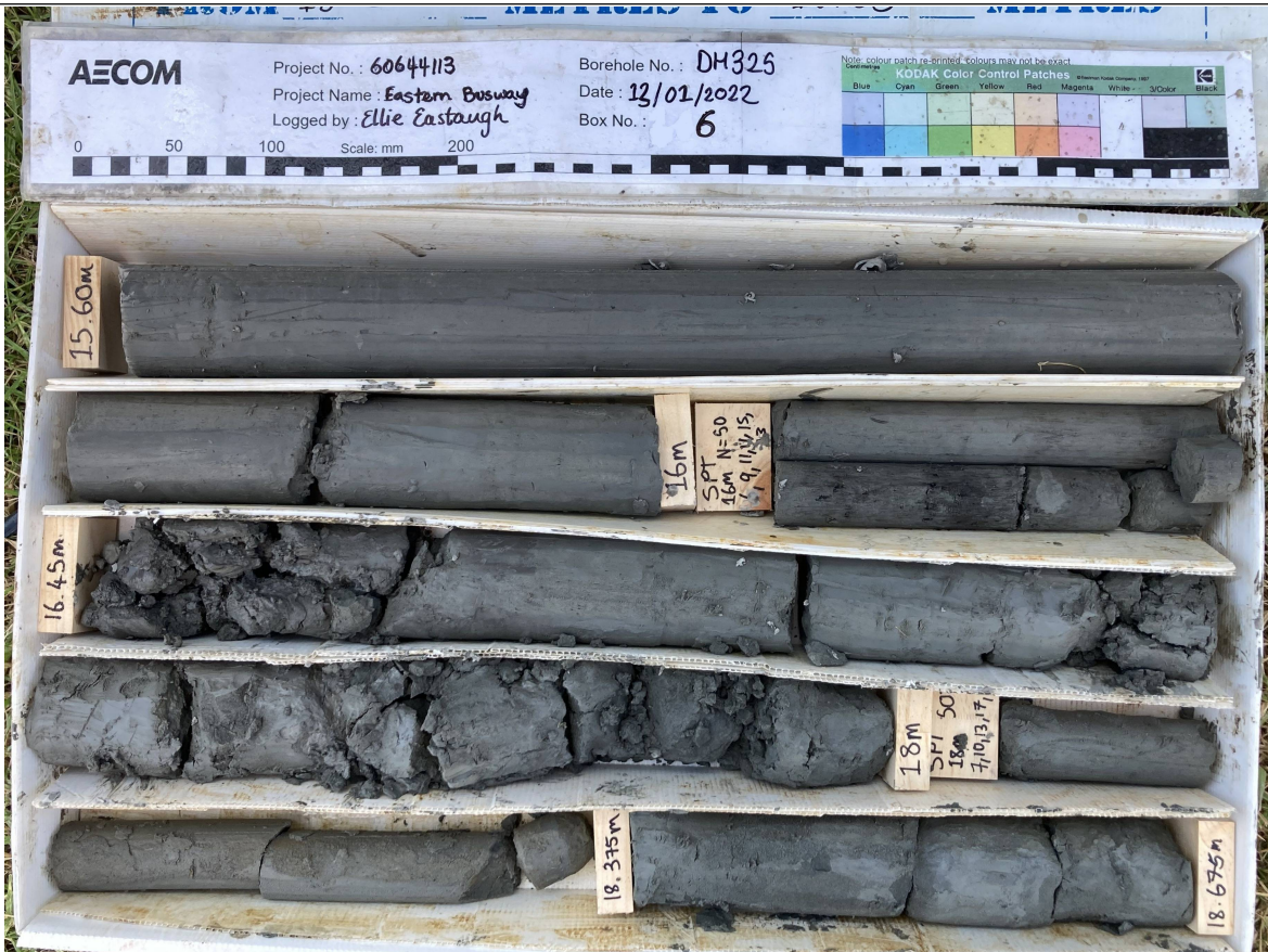
Box: 6 of 9 - Depth: 15.60m to 18.67m of 28.50m Date Drilled 12/01/2022 to 14/01/2022 - Date Photographed: 13/01/2022
